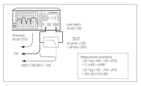
Figure 8. Reflection Example Using a One-Port Cal
