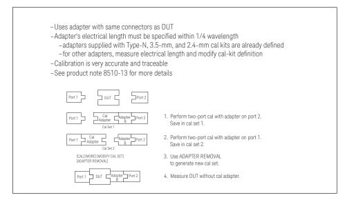
Figure 16. Adapter-Removal Calibration
