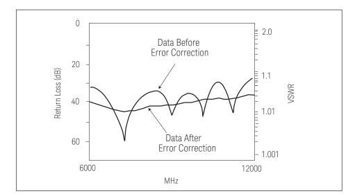
Figure 3. Before and After One-Port Calibration
