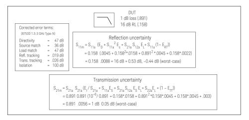
Figure 14. Calculating Measurement Uncertainty after a Two-Port Calibration
