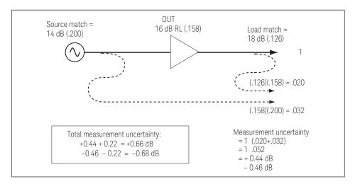
Figure 12. Measuring Amplifiers with a Response Calibration
