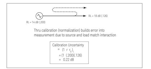
Figure 10. Transmission Example Using a Response Cal
