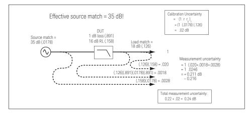
Figure 13. Transmission Measurements using the Enhanced-Response Calibration
