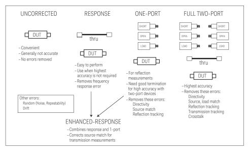
Figure 6. Errors and Calibration Standards
