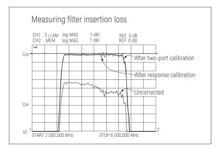
Figure 1. Response versus Two-Port Calibration
