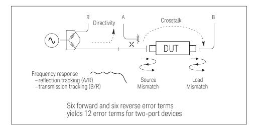
Figure 2. Systematic Measurement Errors
