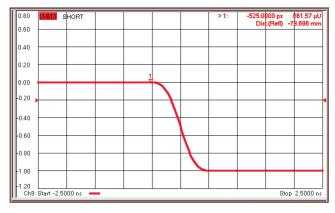
Figure 39. Low-pass step response of a short.
