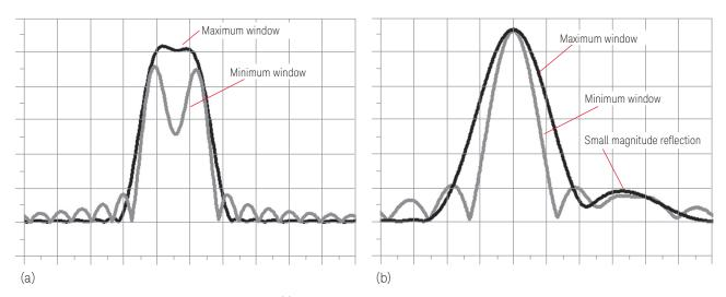
Figure 25. Response changes as window shape changes: (a) minimum window is best when higher resolution is needed to resolve signals with equivalent magnitudes, (b) maximum window is ideal for best dynamic range if responses are very different in magnitude.
