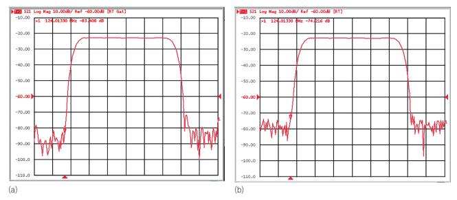
Figure 34. Effect of gating on and off: (a) with gating on, the effect of RF leakage and triple travel signal have been removed, and the result is an improvement in out-of-band rejection, (b) no gating applied (same as Figure 29).
