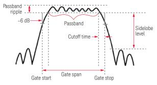
Figure 14. Sample of a gate shape and its parameters.
