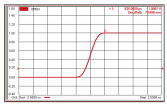
Figure 40. Low-pass step response of an open.
