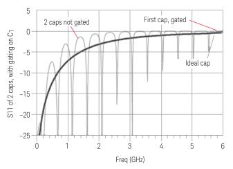
Figure 17. Gating out the first discontinuity (circuit shown in Figure 16).
