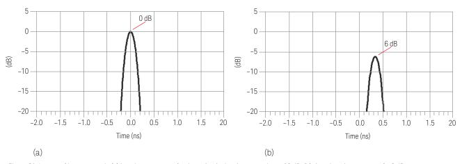
Figure 21. Impact of lossy network: (a) impulse response of a short circuit showing return loss of 0 dB, (b) time domain response of a 3 dB attenuator terminated with a short circuit, 6 dB loss represents the forward and return path loss through the attenuator.
