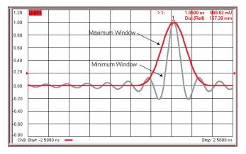
Figure 45. Effect of windowing (minimum or maximum) on an open standard connected to an airline.
