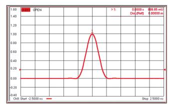
Figure 37. Impulse response of an open standard.
