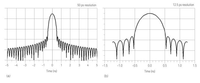
Figure 27. Range resolution: (a) a span of 10 ns results in a range solution of 50 ps, (b) reduce span to 2.5 ns and reduce resolution to 12.5 ps.
