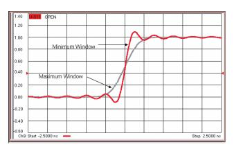
Figure 42. Open standard: the effect of windows (minimum or maximum) on the step response.
