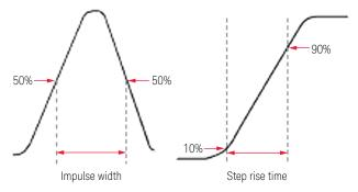
Figure 22. Response resolution is equal to the 50% points of the impulse width or the step rise time of 10 to 90% points.
