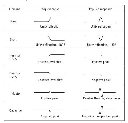
Figure 7. Low-pass responses, both step and impulse, of known discontinuities.
