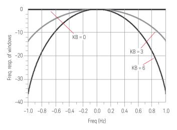
Figure 10. Various Kaiser-Bessel (KB) windows each with a different B value.
