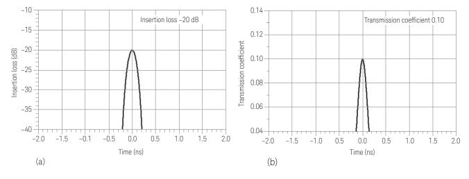
Figure 9. The bandpass response of a 20 dB attenuator displayed (a) in log mag format showing insertion loss in units of dB, and (b) in lin mag format showing transmission coefficient units.
