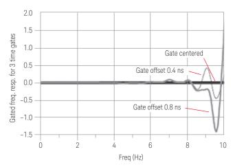
Figure 12c. Frequency response after gating
