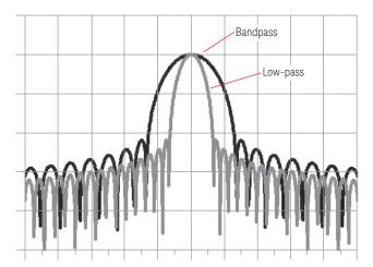
Figure 26. Given the same settings, frequency span and number of points, resolution is different for the low-pass and the bandpass modes.
