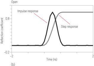
Figure 35. Low-pass responses of a short circuit (a) and an open circuit (b).
