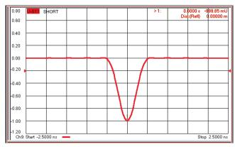
Figure 38. Impulse response of a short standard.
