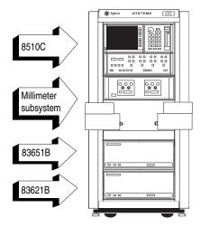
Figure 6. Agilent 8510XF system
