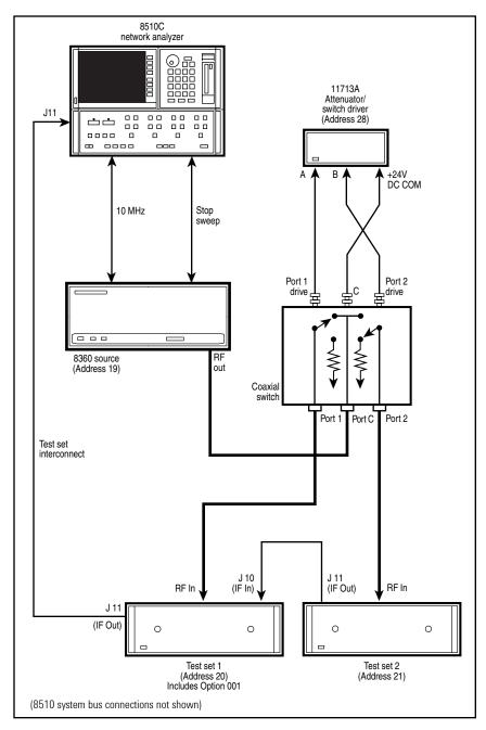
Figure 2. Agilent 8510 dual coaxial test set configuration
